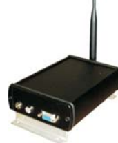
Data transmission speed: 1200...38400 Baud Power supply: 8...12V
