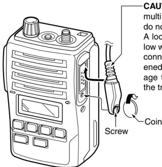
**IMPORTANT:** KEEP the [SP MIC] jack cover attached (transceiver) when the speaker-microphone is not in use. Water will not get into the transceiver even if the cover is not attached, however, the terminals (pins) will become rusty, or the transceiver will function abnormally if the connector gets wet.
