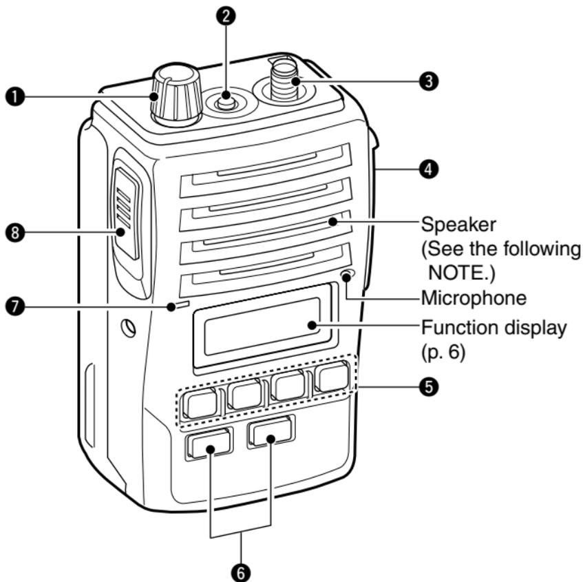
**NOTE:** If the speaker netting (for dust proofing) becomes wet, dry it with a hair drier (cool mode) etc. before operating the transceiver. Otherwise the audio may be difficult to hear for loss of the sound pressure.
