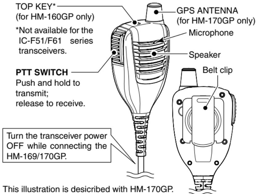
**NEVER** immerse the connector in water. If the connector gets wet, be sure to dry it **BEFORE** attaching it to the transceiver.
