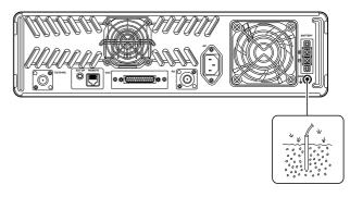
**AWARNING: NEVER** connect the [GND] terminal to a gas or electric pipe, since the connection could cause an explosion or electric shock.
