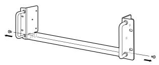
② Remove the handles from the bottom bar. And turn the handles upside down, then replace the handles right side and left side.
