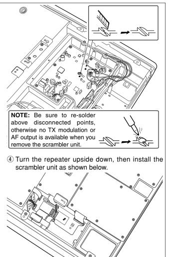
(5) Return the LOGIC shielding plate, top and bottom covers to their original positions.
